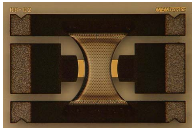
Figure 2 - MEMS capacitive switch fabricated with a molybdenum metal membrane.
